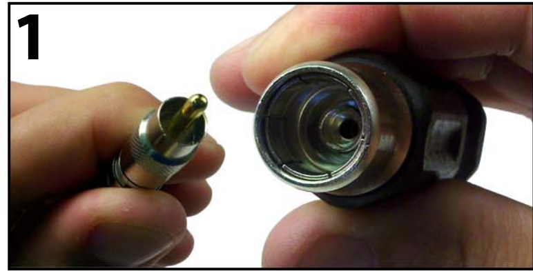
Hold the RCA Connector and CGT-FBR Tool in each hand
