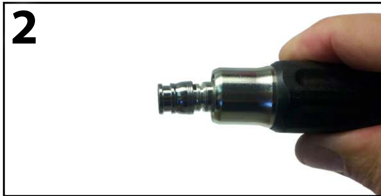
Insert the BNC connector into the large end of the tool
