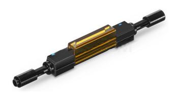
lid without separate installation tool. SelectCom's Optical Fiber Mechanical Splicer is a mechanical splice that provides an inexpensive, quick alternative to mating fibers. Using V-groove technology, this splice maintains physical contact between the fibers. We provide a precise, simple and low cost method of mechanically splicing optical fiber. Fiber can be spliced simply in this way in a very short time. It can be used for 900/900µm, 250/250  $\mu$ m, 250/900  $\mu$ m fibers.
