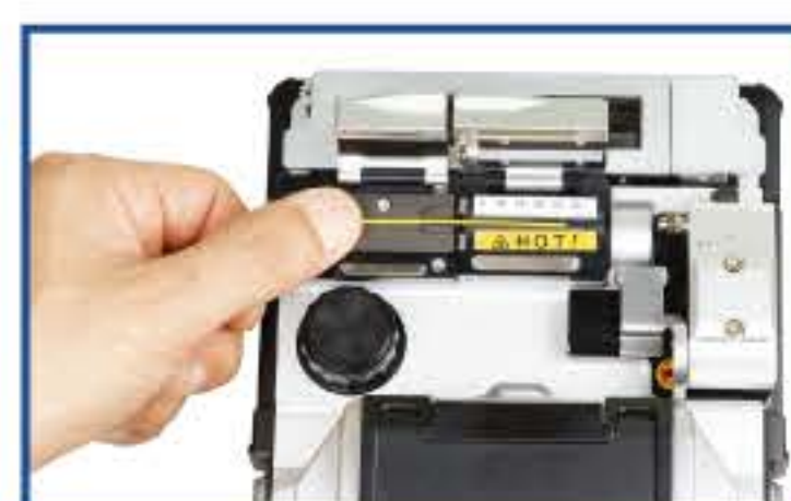
Stripping (No Cracks on Fiber)
